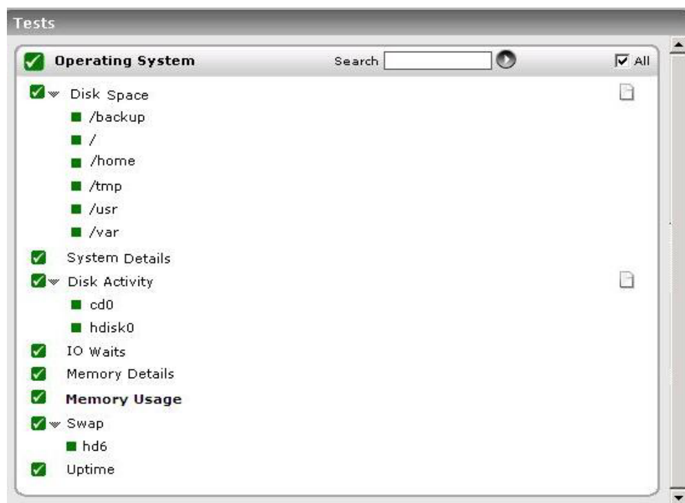
Figure 2.29: Tests that map to the Operating System layer of an HPUX server
