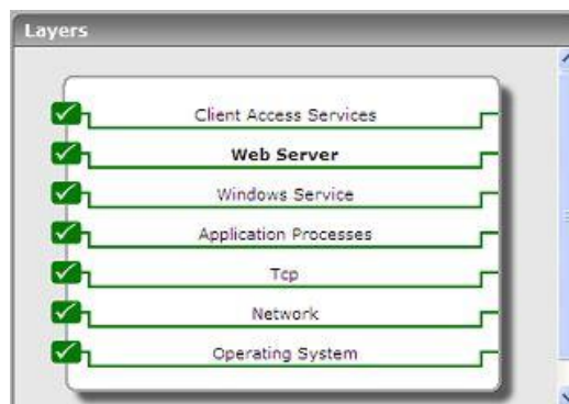
Figure 2.1: The layer model of the Client Access server
