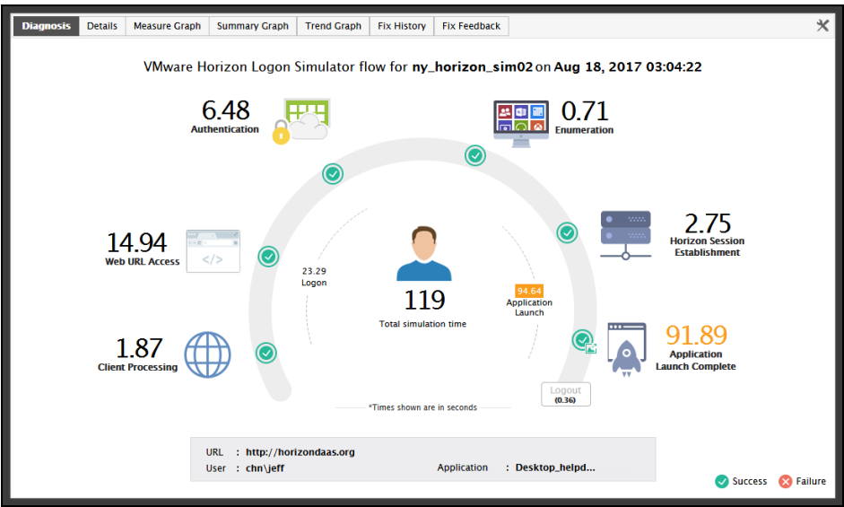
Figure 1.23: The Simulator Dashboard in the eG monitoring console revealing at first glance, the root-cause of logon slowness
